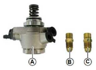
45. Soak with engine oil the seal ring (A) before installing the pump.
