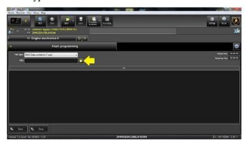
16. Select the VIN of the corresponding vehicle and then click "Open", as shown in the picture.
