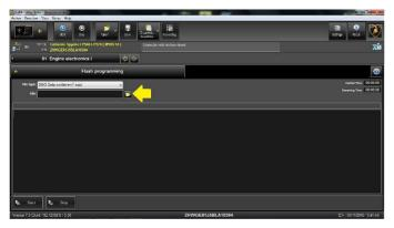
25. Select the VIN of the corresponding vehicle and then click "Open", as shown in the picture.
