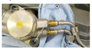
47. Torque the unions (C,D) you have previously installed on the pumps.
