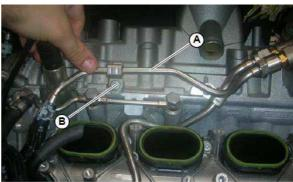
50. Install the mounting (B) of the fuel pressure sensor then fit the new sensor (A). Fasten the fuel lines with the supplied clamps (C).
