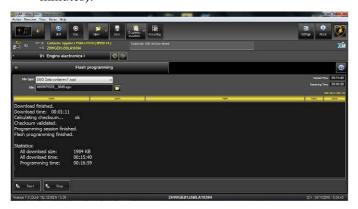
30. When the flash programming of the ECU Engine Master is finished click "OK" and switch OFF the ignition. Wait at least one minute before switching the ignition ON again.
