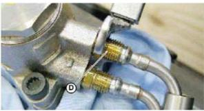
48. Assemble the feed and high pressure lines made of steel. Tighten the nut (G,E) to the pumps (H,F).
