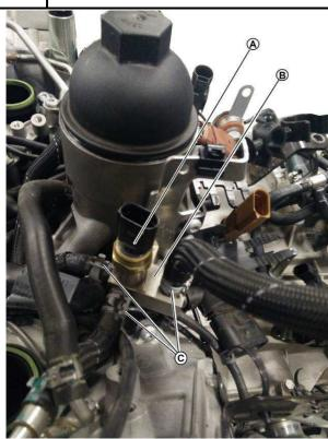
51. Install the feed rubber hoses (A,B,C). fasten the ilnes with the supplied clamps (D).
